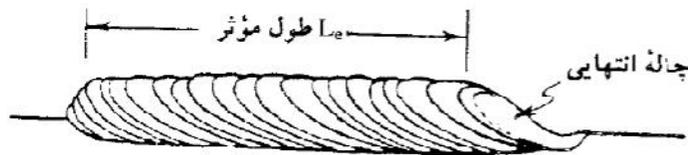
$$L_e \geq 4D \geq 4 \text{ cm}$$
